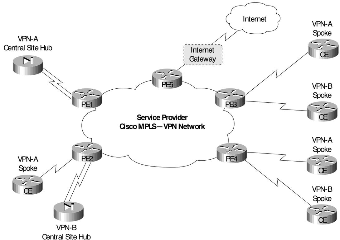
Notice, Internet traffic from any Spoke VPN sites need to pass through a firewall. Since the central site is providing firewall services (as shown in figure 6), a static default route pointing to the central site firewall should be installed in associated FIB tables for each spoke sites.
