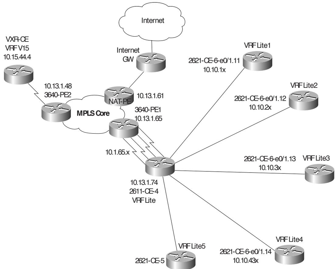
Separate FIB tables are maintained on 2611-CE-4 for each VRFs. Figure 11, shows detailed connectivity information between 3640-PE1 and 2611-CE-4(VRF Lite CE). Notice, there is no separate sub-interface for Internet traffic.
